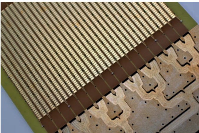
Figure 1 A prototype of the MSA-T antenna array and feed network.
