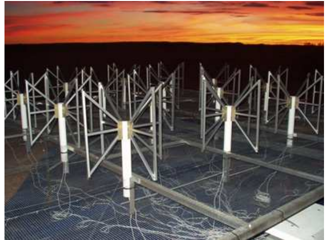
Figure 23: A single antenna tile from the Mileura Wide-Field Array. The final telescope will use dozens of these tiles spread over an area of many square meters. Credit: Frank Briggs (Mt. Stromlo Observatory)
