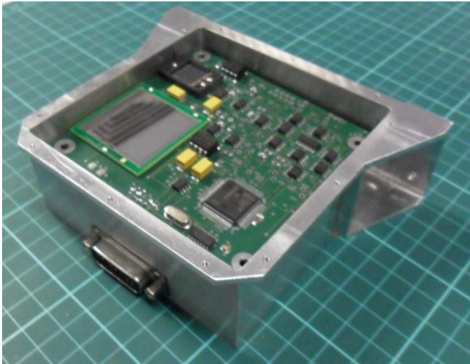
Fig. 1: The MuREM FM unit to be flown on TDS-1 showing the detector board with the two large area PIN diodes to the left of the image.
