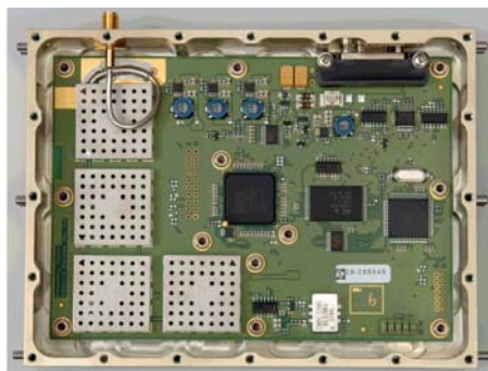
Figure 5: AIS Sensor for AISSat-1.
