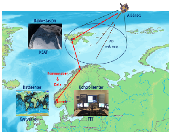
Figure 4: AISSat-1 mission architecture.
