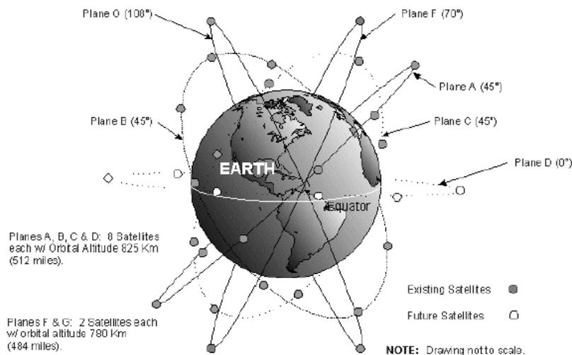
Figure 2 - ORBCOMM System 30 Satellite Constellation including potential positions for 48 satellites
