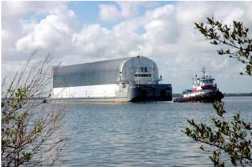
Figure 11. NASA will use the Space Shuttle’s external tank barge to deliver the upper stage IVGVT unit.
