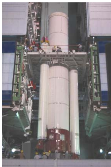
Figure 5. Assembly of S12 strap-on motors in PSLV-C19 at first launch pad.
