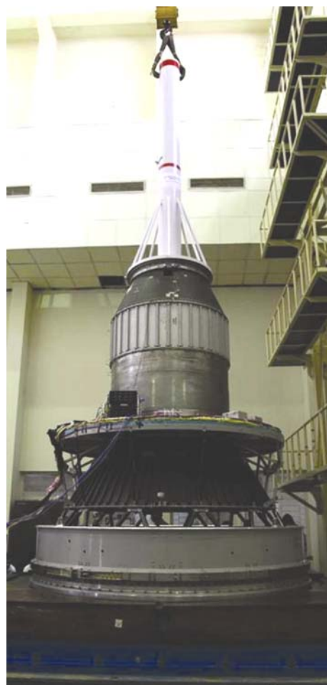
Figure 6. Vibration test of PS4 stage with simulated RISAT-1 mass for dynamic characterization.
