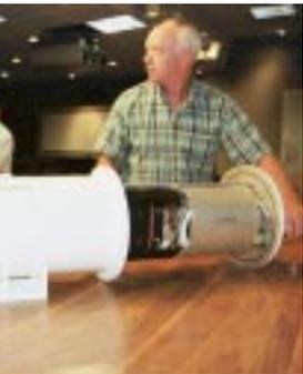
(right) United Space Alliance design engineer, Chris Perri, is shown with a design of housing for a camera which is part of the OTV camera. The camera will be used at the launch pad to detect hydrogen peroxide. (left) is the Dynacs design engineer for the camera housing design was a collaboration between USA and Dynacs. Chris Perri is the lead design engineer for the camera housing design.
