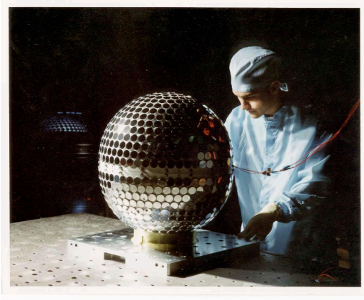
Figure 3 Starshine 1 Satellite on Vibration Table
