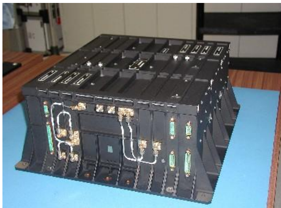
Figure 3 - DORIS DGXX receiver and the on-board antenna
