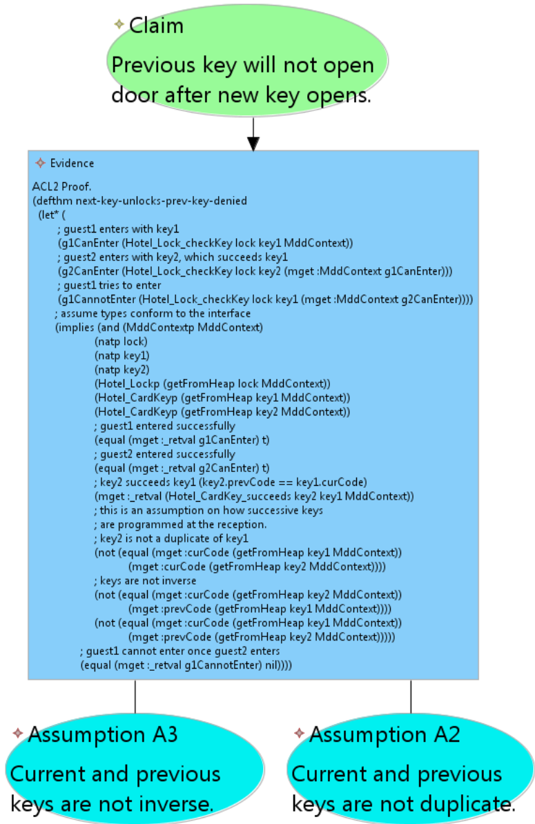
Figure 1 The assurance case fragment for the previous key proof requires two assumptions to be met.
